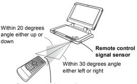
Remote control transmitter Within 7 m (23 ft.) in front
